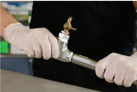
7) Attach the sample valve to the other end of the mixing tube.
