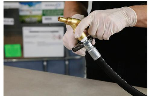
9) Complete the assembly by attaching the fluid gun to the end of the whip hose.
