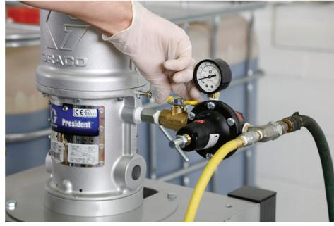
14) Turn the air supply to the air motor pump on.
