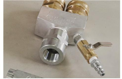
3) Remove the manifold head, mixing components and fluid gun from the solvent container and wipe off any excess solvent with a dry rag. Visually check to ensure all items are free of residue.
