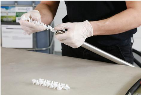
4) Position the mixing tube with the tapered end down and insert the flat end of the first element into the mixing tube stopping one inch from the top. Insert the next element into the notch of the first element and push down. Repeat for the remaining elements. 3/4 inch mixers require four elements. 1/2 inch mixers require three.
