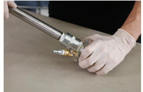
6) Attach the mixing tube to the coupler on the manifold head and tighten.
